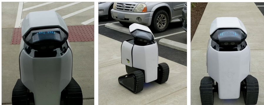
Fig. 2. Cropped frames from the online survey-based study stimulus videos. From left to right: the “delivery” stimulus, where the robot approaches, stops, and then opens its compartment; “passing”, where the robot passes by, tilts its head, and makes a happy facial expression; and “stopping”, where the perspective walks in front of the robot, blocking it and causing it to shake its head and make an unhappy facial expression.
